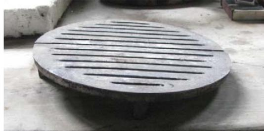
The slots may not be wide enough or the top not round enough. It did not perform as well as the grate made from round steel bars – it produced much more charcoal. The best shape for the top of the bars may be cylindrical, not flat.
