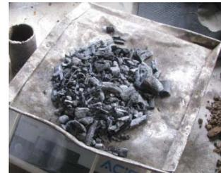
3.3.3. The photos at the right show the effect on char production in an SAE Stove and an SAE Stove (next page) with the same grate fitted (below). It also has a flat-bottomed combustion chamber and received the same benefit when the grate was added.
