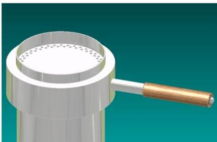
A wire mesh dome is then placed on top of the burner housing (picture on right). The dome immediately turns red hot and emits electromagnetic waves.<sup>3</sup>
