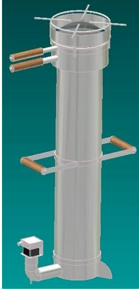
The gasifier seen here is nothing more than a vertical cylinder with a removable burner on top and a grate at the bottom. A small fan supplies air underneath the grate, and the speed of the fan is controlled by means of a speed regulator. On a given biomass and at a given fan speed, the diameter of the reactor determines the amount of gas produced, and the height of the reactor determines the length of time that this gas is produced.
