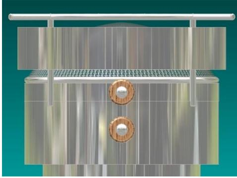
The flames closely follow the contour of the dome. At the base of the dome, additional secondary air is drawn in to complete the combustion of gases. The dome gives structure to the flames and protects them from the wind. The wire mesh dome also filters out cinders and other fine particles that are emitted by the reactor. It is absolutely imperative that the operator of the gasifier not inhale these fine particles.<sup>4</sup>
